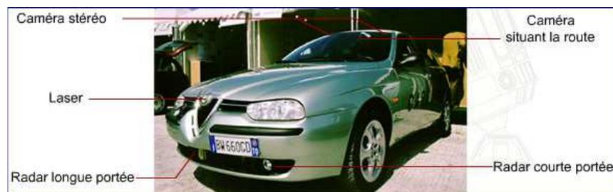
FIG. 1.3 – Le prototype Carsense.
